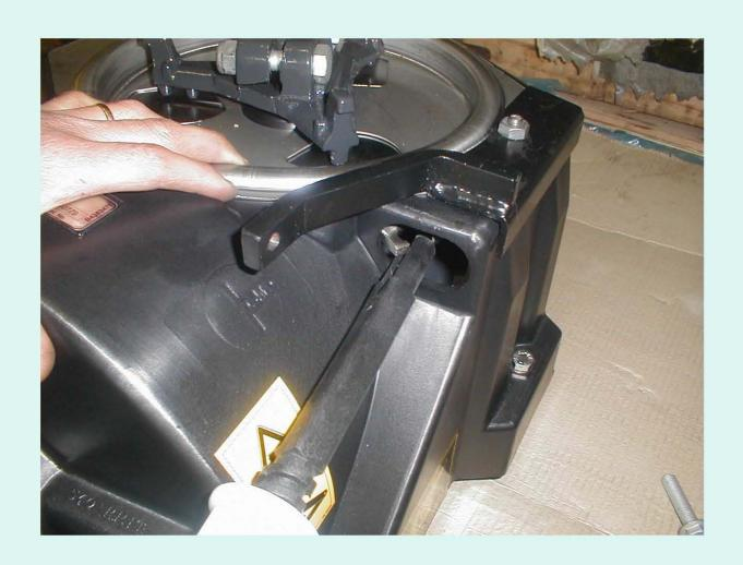
Fix the pto shaft protection cover by three self-threading screws.
