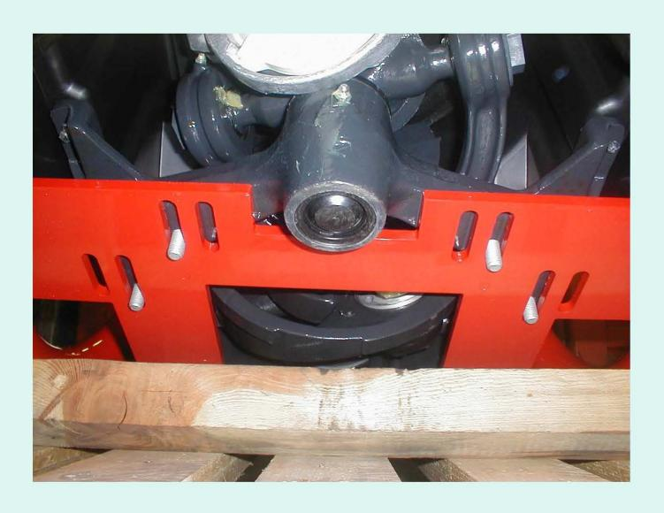
Put the rectangular tube for hopper support and its rods.
