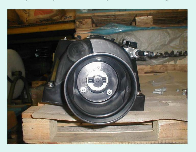
Put four bolts into the gear box's holes. Attention! The longer two bolts must be inserted towards the pendulum.
