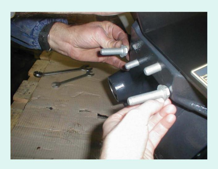
Put the gear box on the frame and fix it without tightening bolts and nuts.
